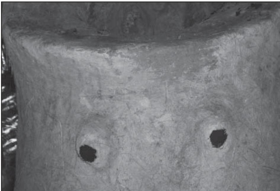
**Figure 6.** Wollega (west) furnace which is spectacularly built in a house is of over 60 cm diameter at the bottom. This allows them to enter through the bottom aperture in order to plaster its inside. Note a man is seen sitting inside the furnace while the other is providing him with clay plaster. The aperture is not sealed off until the day of the smelt.
